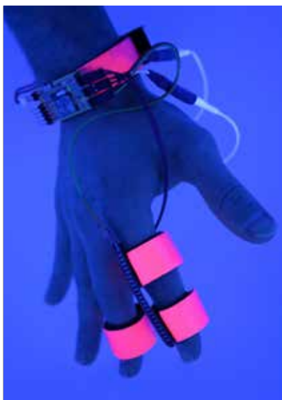
THE DORMIO glove (above) can sense when its wearer dozes off (below). It then shares audio cues to influence dream content.
